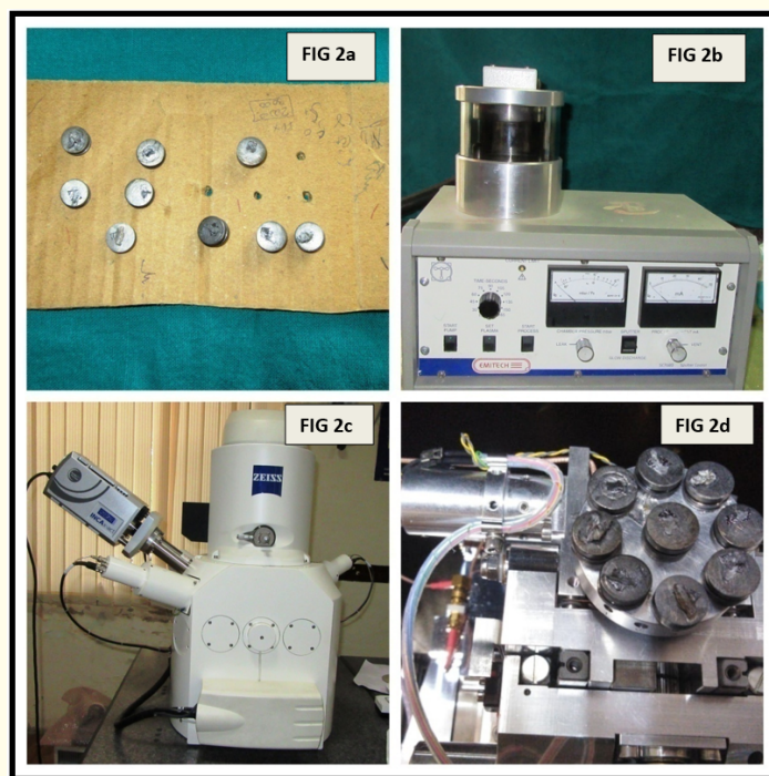
Figure 2: 2a: PRF samples loaded on to aluminium stubs. 2b: Gold sputter coating machine. 2c: Scanning electron microscope. 2d: PRF samples after gold sputtering placed into the SEM chamber.
