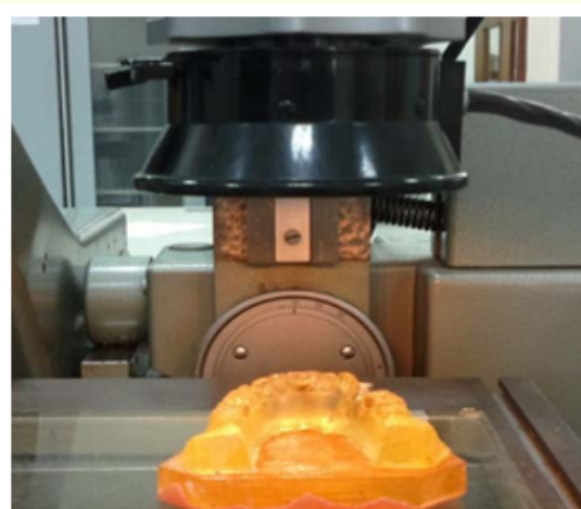
Figure 7: Top view of master model under the traveling microscope.
