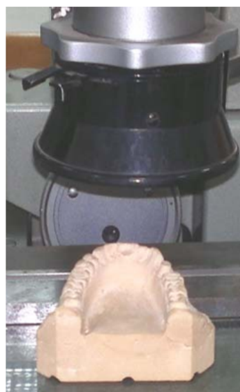
Figure 13: Improved stone cast under the traveling microscope.
