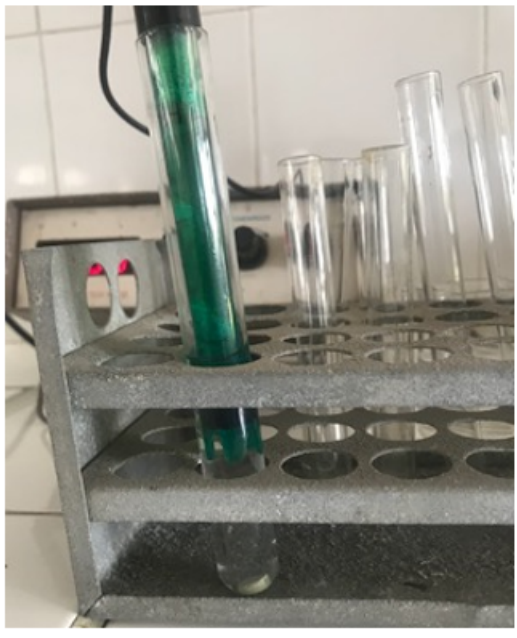
Figure 3: pH meter inside the test tube containing sample.
