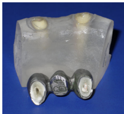
Figure 4: Cervical fracture of endodontically treated teeth when used as abutment in FPD without posts [21].
