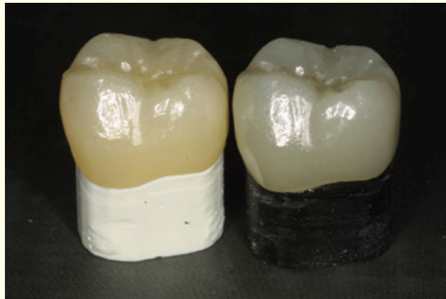
Figure 3: High translucency of ultra-translucent ceramic seen placed on a black and white dye [15].
