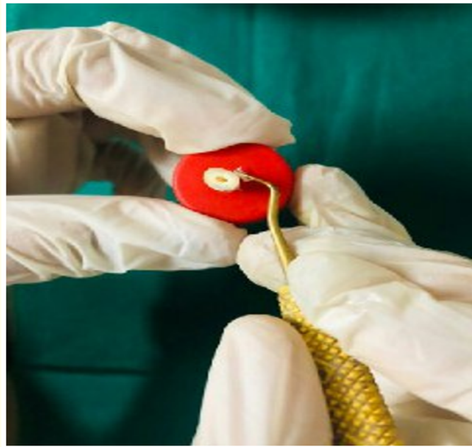
Figure 2: Gap between the tooth and the lid sealed with Filtek Z250 Composite resin.
