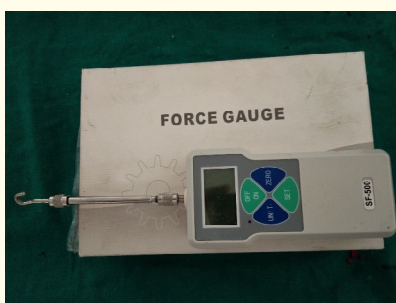
Figure 8: Digital force gauge.
