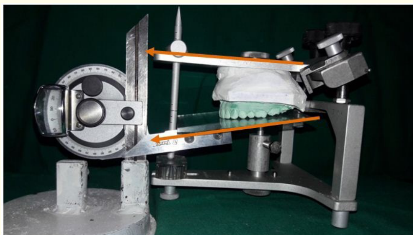
Figure 8: Angle measurement on Whip mix articulator.
