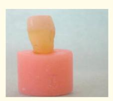
Figure 3: Embedding of teeth in the acrylic molds.
