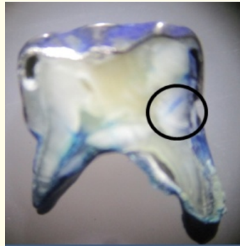
Score 2: Dye penetration more than 1/3rd but till 2/3rd or less from the prepared outer surface.
