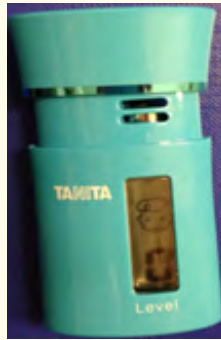
Figure 1: FitScan Breath Checker: the device in operational mode, objectively determining the degree of bad breath.
