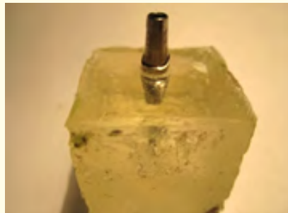
Figure 1: Epoxy resin block with titanium abutment.
