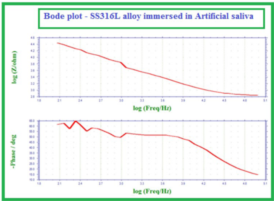
Figure 14: AC impedance spectra (Bode plot) of SS 316L alloy immersed in AS.
