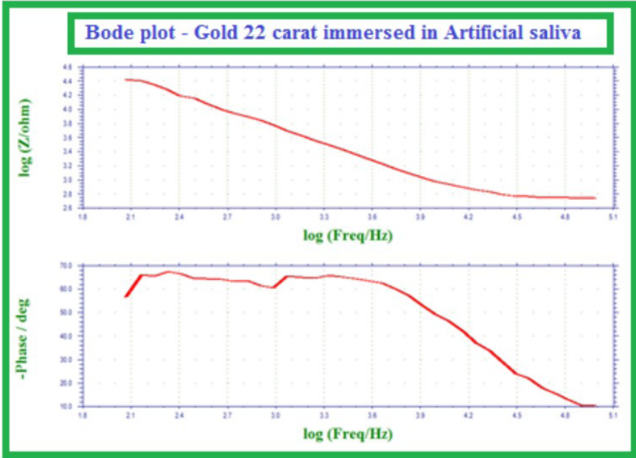
Figure 6: AC impedance spectra (Bode plot) of Gold 22 carat immersed in AS.
