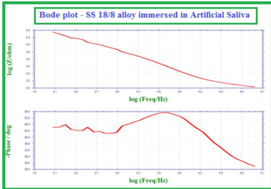
Figure 10: AC impedance spectra (Bode plot) of SS 18/8 alloy immersed in AS.
