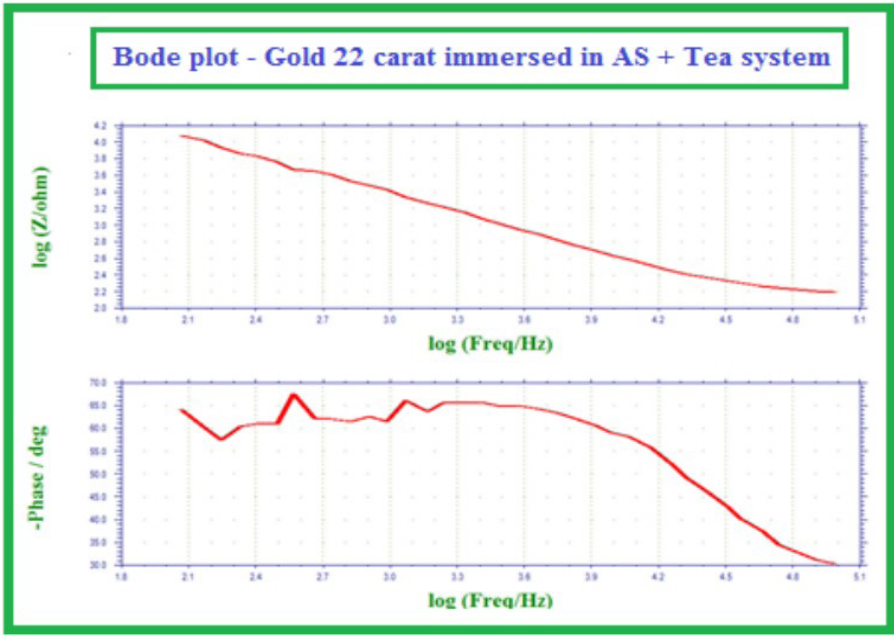
Figure 8: AC impedance spectra (Bode plot) of Gold 22 carat immersed in AS + Tea.
