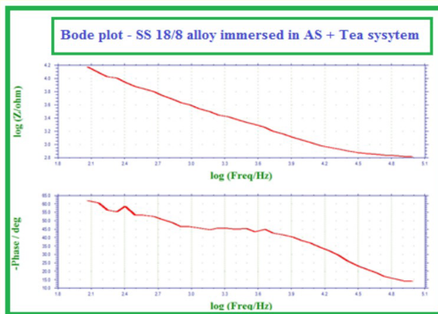
Figure 12: AC impedance spectra (Bode plot) of SS 18/8 alloy immersed in AS + Tea.
