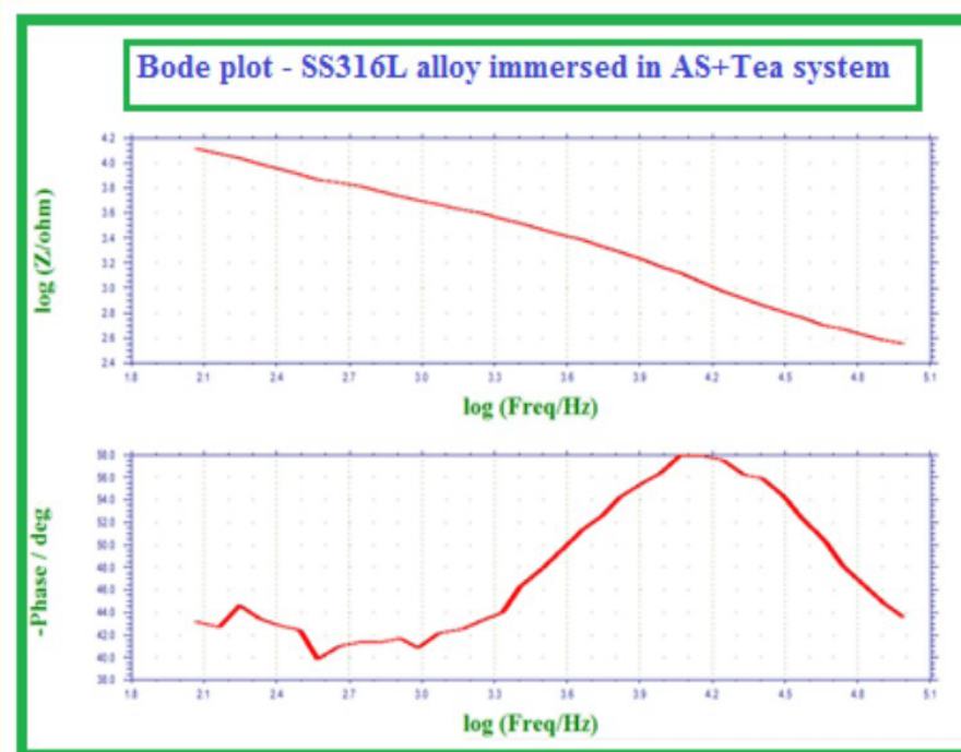
Figure 16: AC impedance spectra (Bode plot) of SS 316L alloy immersed in AS + Tea.
