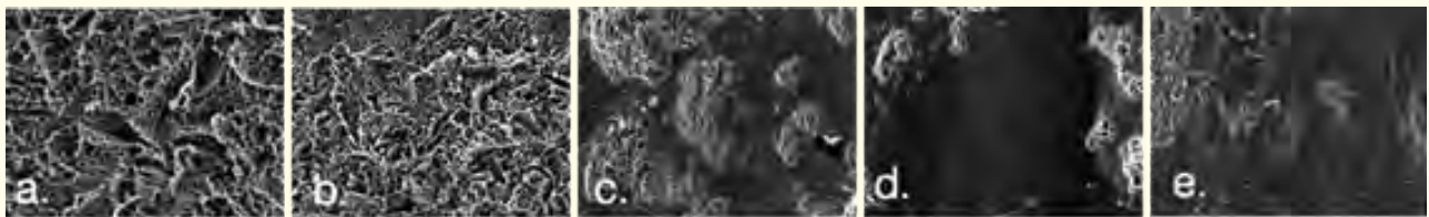
Figure 2: SEM images at 600x after 1 min. of treatment: a) untreated control implant showing no surface damage; b) TiBrush; c) TUS; d) SSC; e) CUS.
