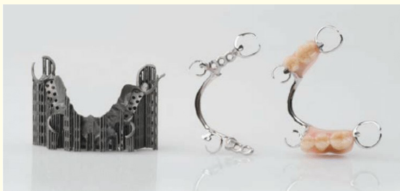
Figure 2: Stages of production for a laser sintered removable partial denture: Dental prosthesis directly after manufacturing, with support structures removed and surface polished, after completion (left to right-Image courtesy of EOS GmbH) [4].
