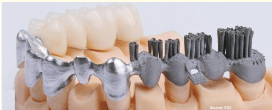
Figure 3: Image shows the progression from 3D Printed framework, to polished part, and then finally veneered finished product. Note the rectangular tracking tag that holds the serial number identifying each part [4].
