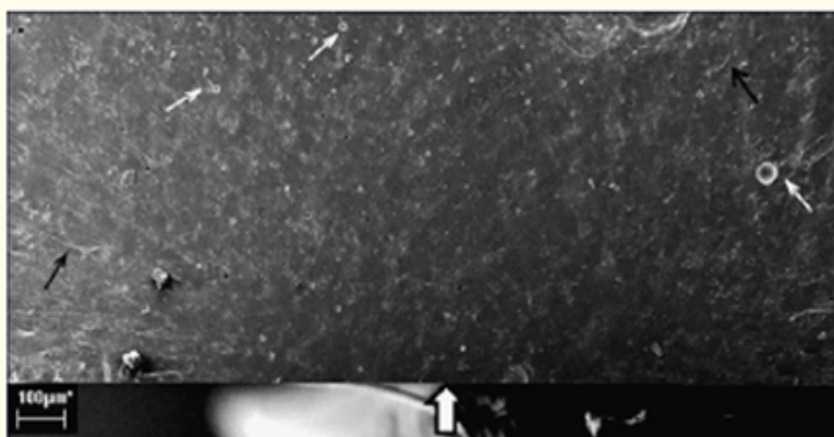
Figure 3: An example of a fractographic analysis conducted based on SEM image. Thin arrows indicate the hackles formed during the fracture process occurring in the ceramic material (Sgura R., et al. Journal of the Mechanical Behavior of Biomedical Materials , 2012).
