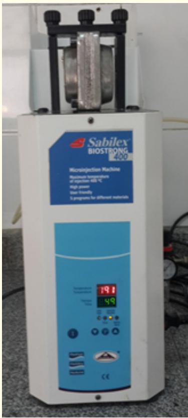
Figure 3: An electric cartridge furnace (Sabilex BIOSTRONG 400). The cartridge is aligned with the flask opening.
