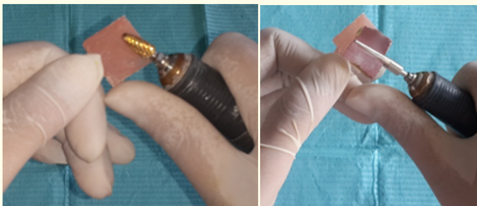
Figure 5: Finishing with tungsten carbide bur and then by sand paper.
