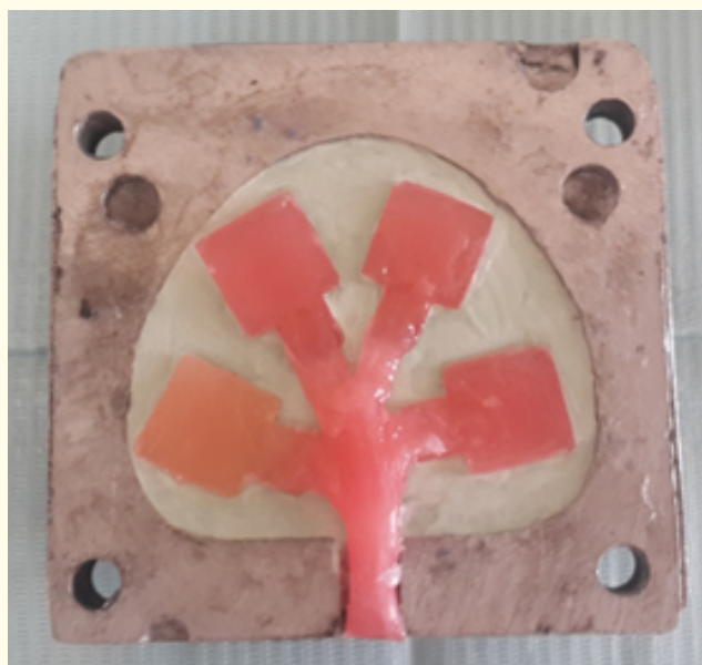
Figure 1: Each wax specimen was attached to sprue then the four sprues were united to form one common sprue. The surface of the wax and dental stone was coated by separating medium.
