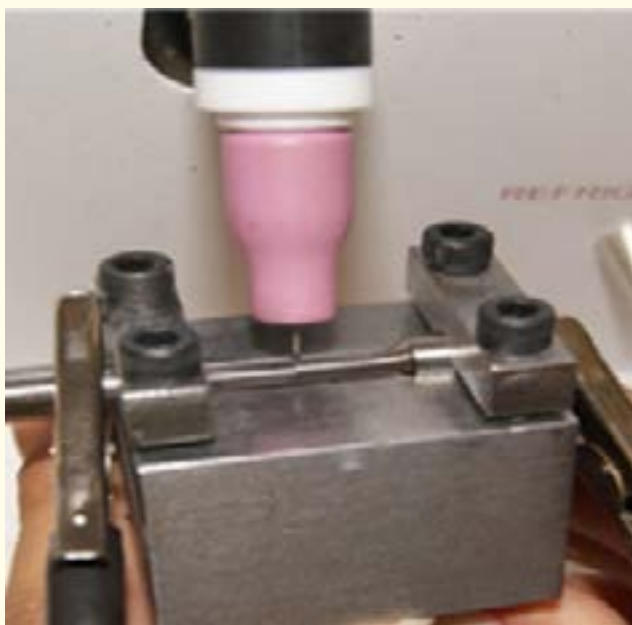
Figure 5: Ceramic torch, with tungsten electrode, positioned over the sample.
