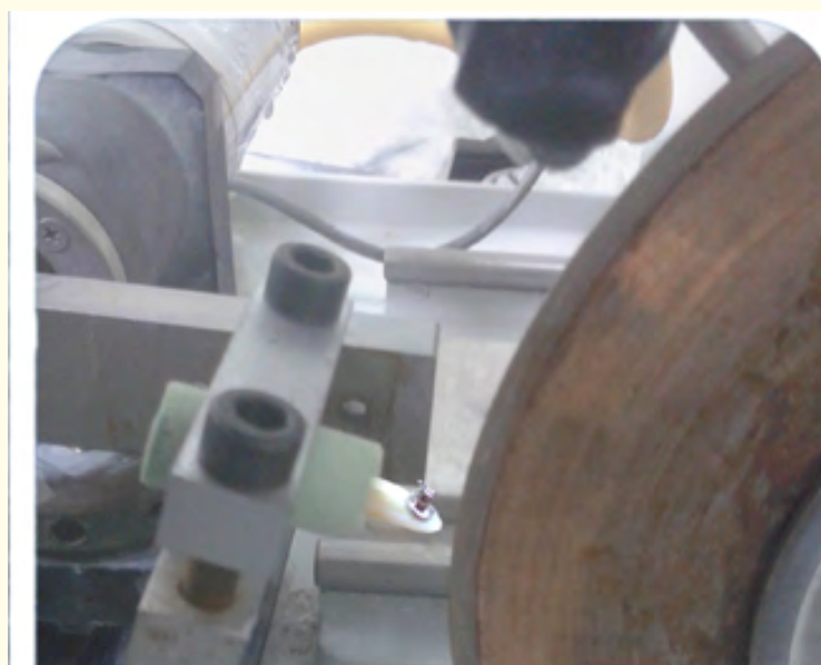
Figure 6: Metal disc used to cut the specimen for microscopic examination.
