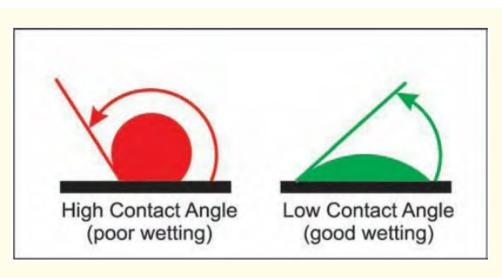
Figure 1: Contact angle measurements demonstrate a liquid's ability to wet a surface.
