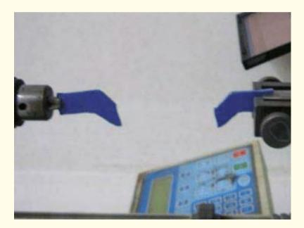
Figure 11: Specimen after complete tearing.
