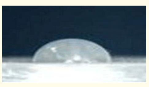
*Figure 13:* Captured photo for the wetting solution drop on the surface of horizontally fixed *TR sample.*
