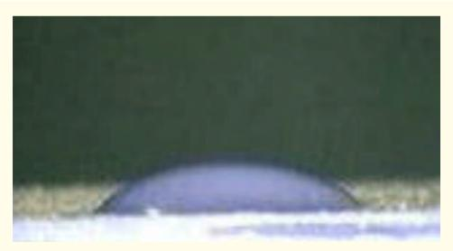
*Figure 14:* Captured photo for the wetting solution drop on the surface of horizontally-fixed VSE sample.
