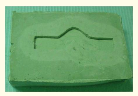
*Figure 6:* Un-nicked 90-degree angle shaped specimens according to American Society for Testing and Materials (ASTM) No.D624-911 for tear strength testing.
