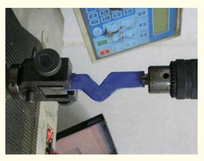
Figure 10: Tear strength testing of vinylsiloxanether.
