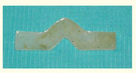
Figure 7: A specimen of thermoplastic resin.
