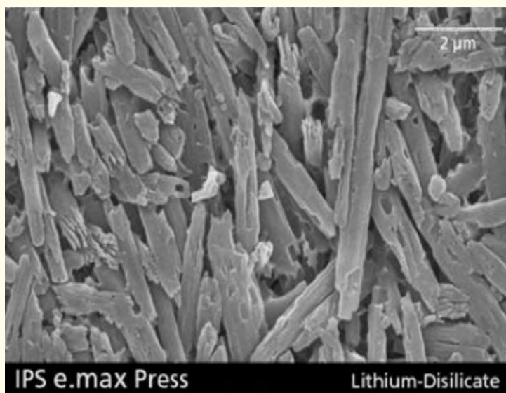
Figure 1: Microstructure of IPS e.max Press (SEM, etched with HF vapour for 30 s).
