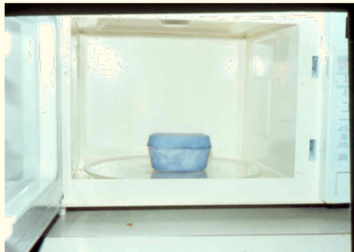
Figure 6: Packed stone mold inside microwave oven during curing.
