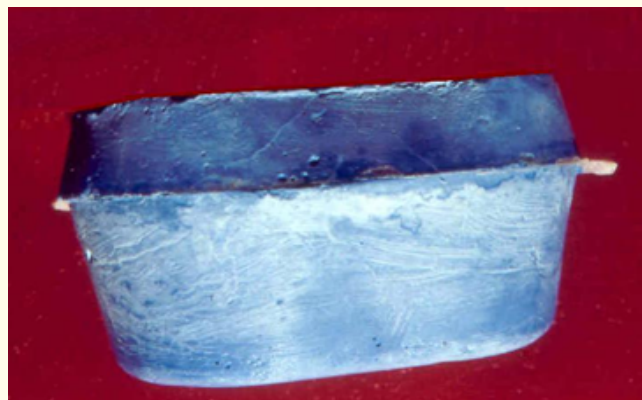
Figure 5: Retrieved stone mold from metal brass flask ready for microwave curing.
