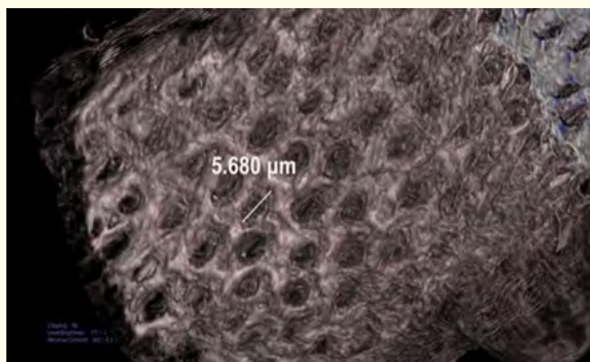
Figure 7: Close-up view of the volume rendering image obtained from SR X-ray CT data. This image is from group A and the white scale bar spanning one patent tubule corresponds to 5.68 μm.
