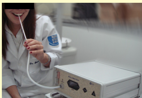
Figure 2: Halimeter employed in the research. Participants with his mouth half open, waiting for the halimeter register the highest result of sulfides in ppb.
