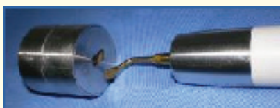
Figure 4: Torquimeter key used for final pressure of the ultrasonic insert deadlocking.
