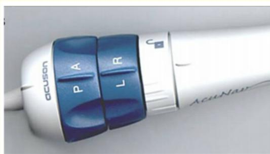
**Figure 1:** AcuNav Catheter. The control handle has three knobs: first to move the tip in posterior/anterior directions, second to move the tip in right/left directions, and the last knob is a locking one that will fix the tip in the desired orientation.
