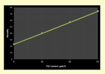
Figure 4: Relationship between Viscosity and PVC content.
