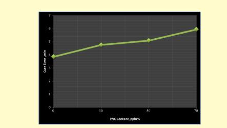
Figure 3: Relationship between cure time and PVC content.
